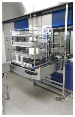
Thanks to one loading and unloading point, staff no longer has to push around the carts between four washer-disinfectors.
