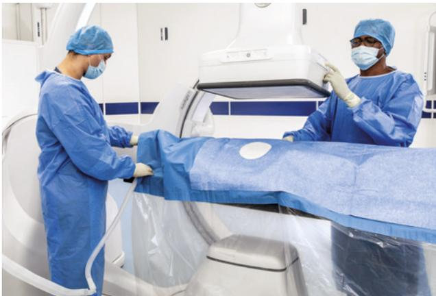
Longitudinal and lateral shift can all be adjusted via the buttons of the Allia detector, allowing more control from different operator's position.
